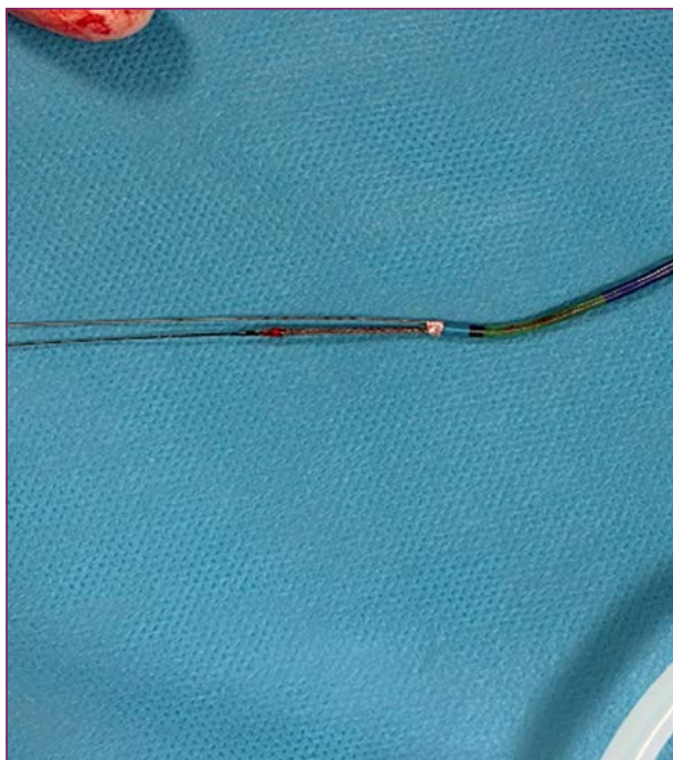
Figure 1. Ex vivo appearance of the retrieved stent-balloon system. Separation of the proximal segment of the stent from the balloon, balloon perforation, and stent deformation at the tip of the guiding catheter are clearly observed.
